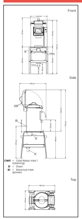
Electric Supply voltage: 603515 (DT15E1C) 220-240 V/1N ph/50/60 Hz 200-240/380-440 V/3 603516 (DT15E324C) ph/50/60 Hz Electrical power, max: 0.37 kW 0.37 kW **Total Watts:** Capacity: Performance (up to): 240 kg/hour Capacity: 15 litres Key Information: External dimensions, Width: 440 mm External dimensions,
